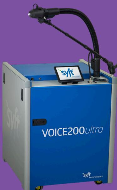
The high sensitivity, high selectivity, real-time analysis, and low maintenance requirements of Syft Technologies' SIFT-MS solution provides reliable and rapid detection of diverse AMCs, minimizing damage to equipment and product.
